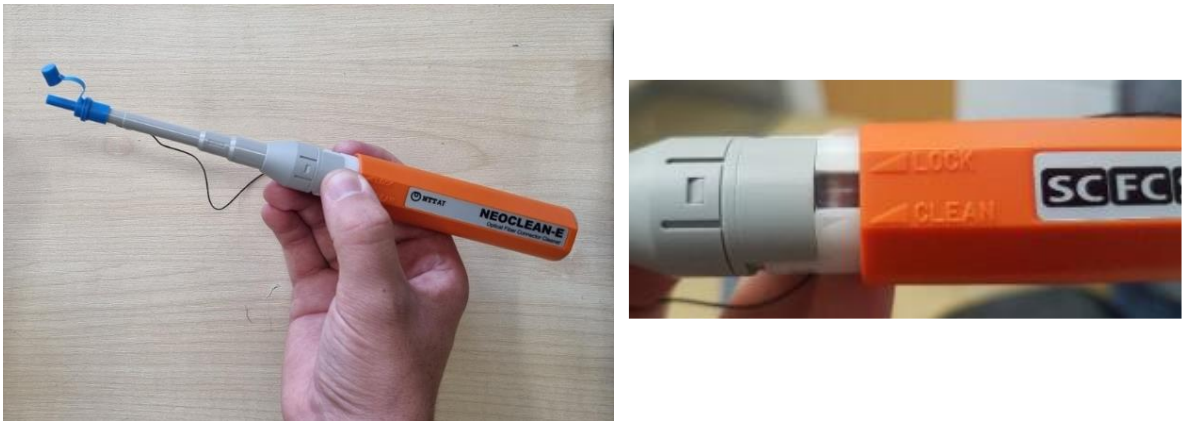
Figure 7. Preparing the Neoclean-E Optical Fibre Connector cleaner.
