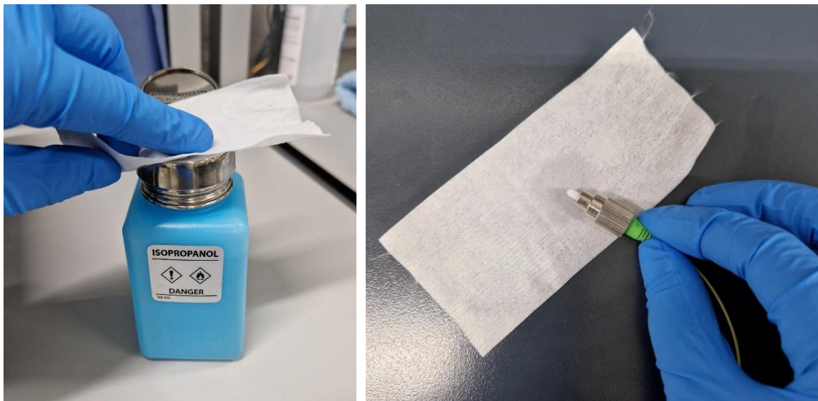
Figure 10. Cleaning the connector ferrule using IPA and a lint-free clean wipe.
