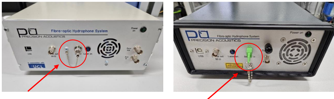
Figure 3. Removing the dust cap from the 'Sensor In' adaptor.
