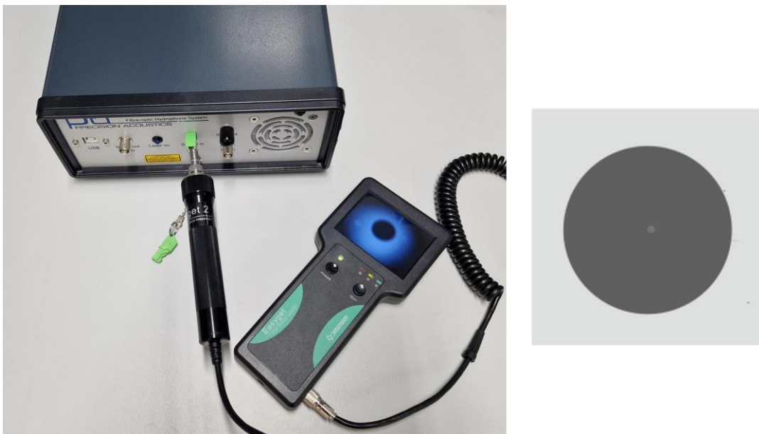
Figure 5. Inspecting the fibre-optic hydrophone system 'Sensor In' using the EasyGet2 portable fibre endface inspector.
