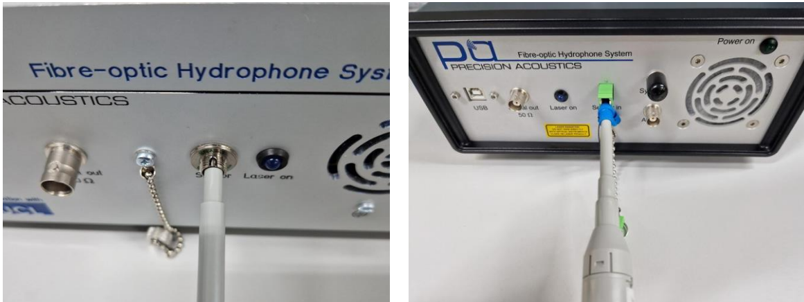
Figure 4. Cleaning the fibre-optic hydrophone system 'Sensor In'.
