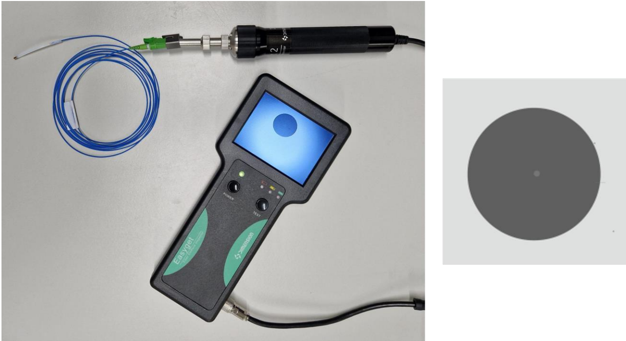
Figure 9. Inspecting the sensor optical connector ferrule using the EasyGet2 portable fibre endface inspector.
