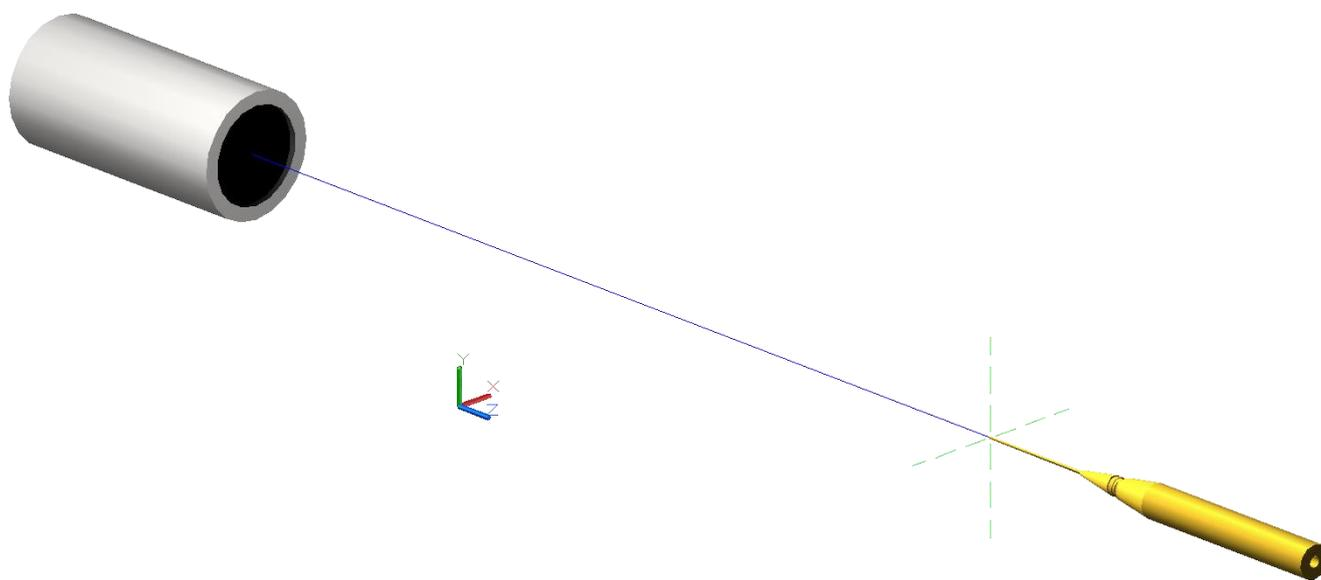
Figure 4 – Orientation of needle hydrophone during use
