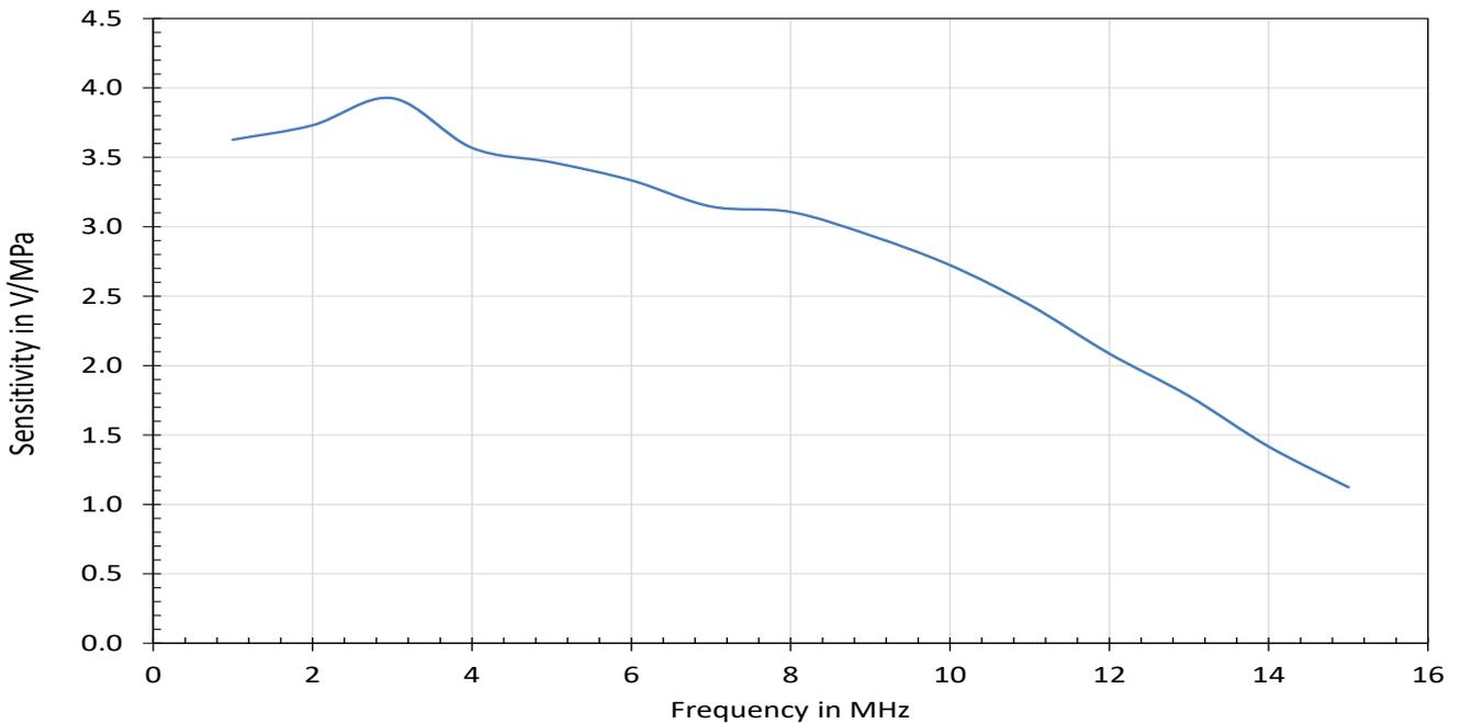
Figure 3 - Typical frequency response of a 2.0 mm needle hydrophone in the range 1.0 MHz to 15 MHz
