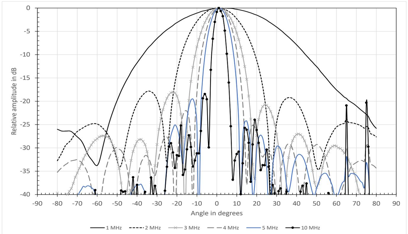
Figure 5 – Directional response of 2.0 mm needle hydrophone
