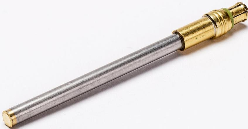
The 2.0 mm needle hydrophone is one of a range of needle hydrophones manufactured by Precision Acoustics Ltd. It is designed to be used in conjunction with a submersible preamplifier and DC coupler with power supply to form a hydrophone system. Whenever properties are reported in this data sheet they refer to those of a hydrophone system incorporating a 2.0 mm needle hydrophone, preamplifier and DC coupler.
