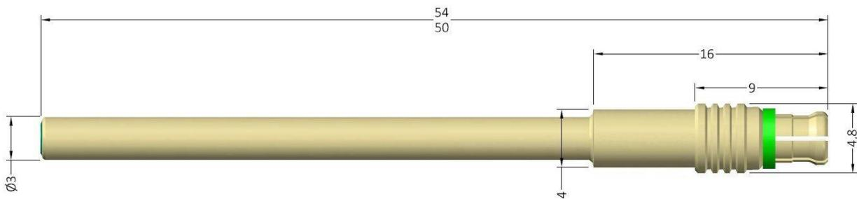
Figure 1 - Dimensioned drawing of 2.0 mm needle hydrophone (NH2000)
