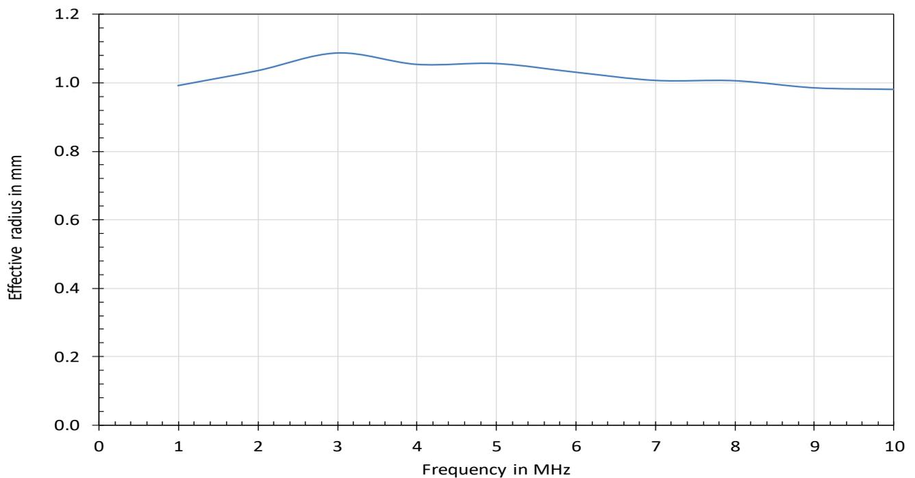
Figure 6 – Effective radius of 2.0 mm needle hydrophone
