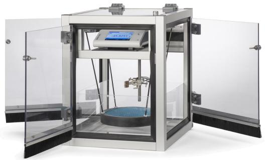
A Radiation Force Balance (RFB) provides a means to directly measure the power produced by a source of ultrasound. It accomplishes this by means of a highly accurate micro-balance that is used to determine the acoustic radiation force that occurs when ultrasound is incident upon a highly absorbing target. The RFB from Precision Acoustics Ltd can be used to measure ultrasonic power from 10 mW to 100 W over a wide range of frequencies.
