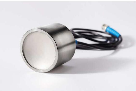
High intensity focussed ultrasound (HIFU) sources are entirely undamped devices designed to produce maximum possible output.
