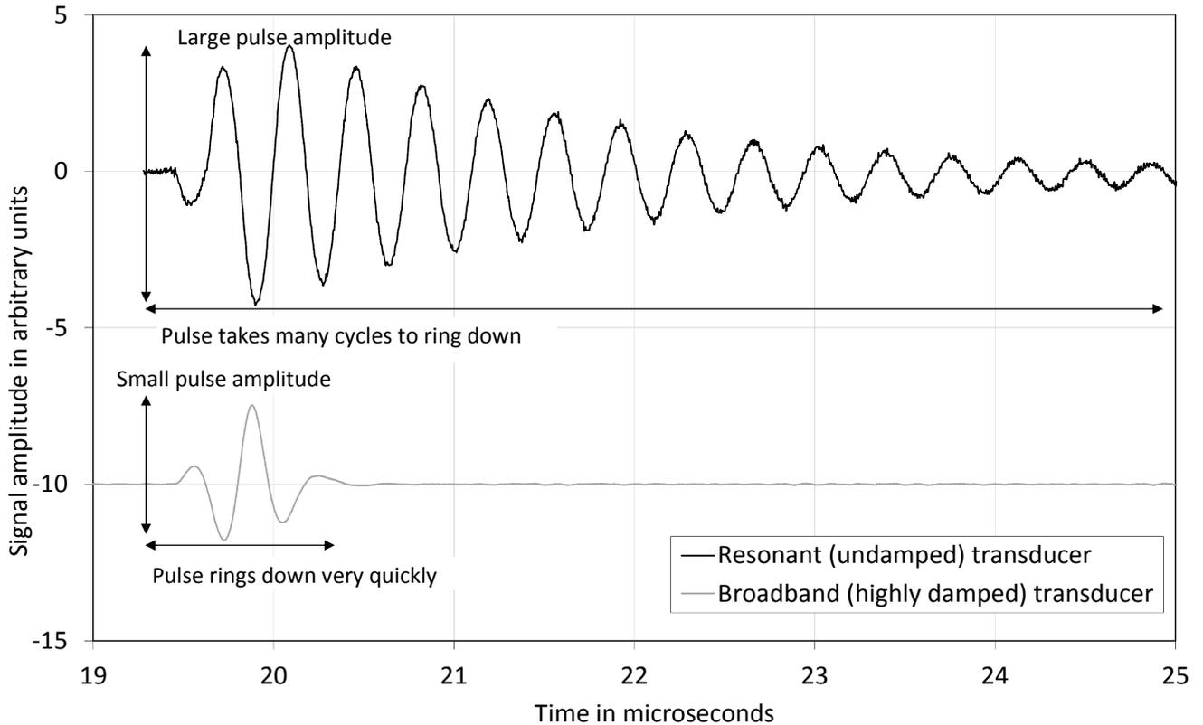
An undamped (or resonant) transducer will produce a large output very close to its resonant frequency, but the amplitude of its response will decrease significantly away from the centre frequency. In contrast a highly damped transducer will produce a much lower output, but is capable of driving at a range of frequencies either side of the centre frequency.
