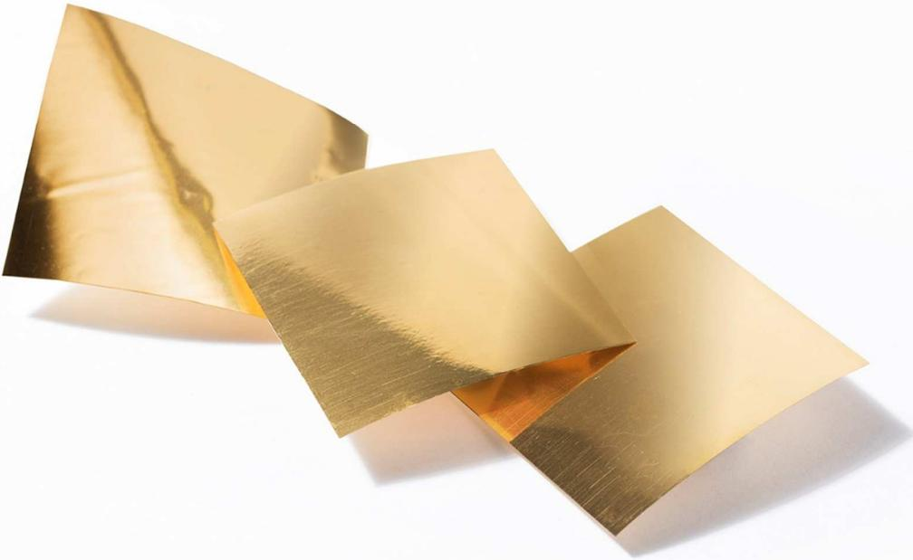
The PVDF student kit comprises 3 pieces of uniaxially poled PVdF each with electrodes of 250 nm Gold on top of 40 nm Chrome. There will be some small scale variation in poling and therefore all data is an indication of properties and cannot be guaranteed.
