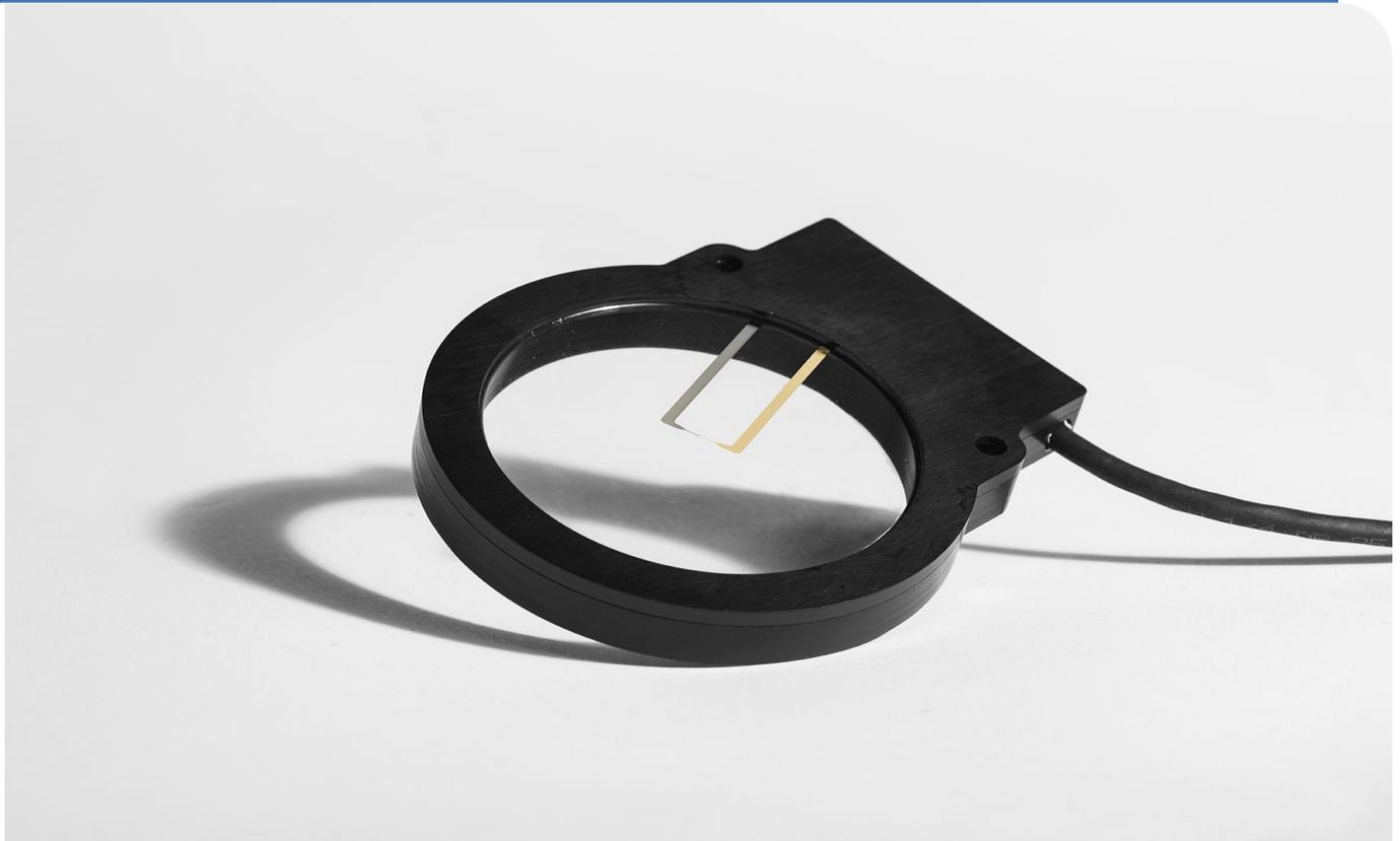
The 0.4 mm differential membrane hydrophone is one of a range of membrane hydrophones manufactured by Precision Acoustics Ltd. It is designed to be used in conjunction with its own dedicated power supply to form a hydrophone system. Whenever properties are reported in this data sheet they refer to those of a hydrophone system incorporating a 0.4 mm differential membrane hydrophone and power supply.
