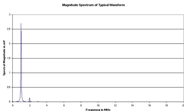
Clearly in this case the frequency spectrum is dominated by the 1MHz component, but the 2MHz component is still clearly visible. As a first approximation, for this waveform, we could neglect the contribution from components other than 1 MHz. This would serve to simplify our calculations, at the expense of a little accuracy.
